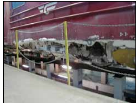
Headache. Before the installation of the Nordic systems. A local train out of service because of ice.
