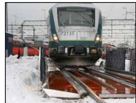
Anti-icing treatment as a final measure before the train goes into traffic.
